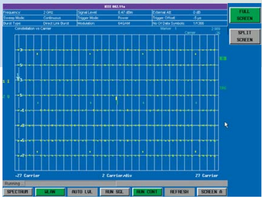
FIG 6: Constellation overview of all carriers; single-carrier constellation is vertical; I and Q values have different colours. This diagram gives a quick overview of all carriers.
